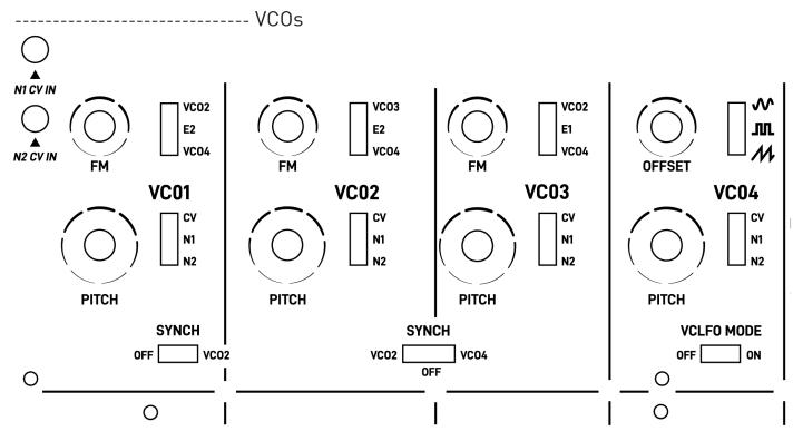
Three VCO are sine wave, the fourth is wave selectable (sine, square, saw) VCO1 and VCO3 are hard syncable via the SYNC switch.
