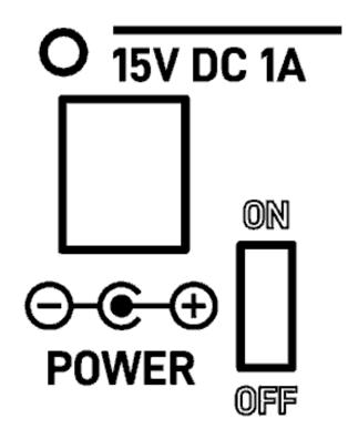
ARPOLOOP works with 15 Volt 1A power supply, center positive, there is a reverse polarity protection and a fuse to secure operation.
