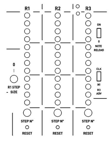
RAMP generators (R1,R2,R3) are driven by the clock pulses and generate a stepped voltage that is displayed by the three led strips the number of steps is controlled by the STEP N. knobs.
