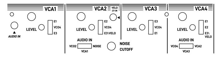
Each VCA is connected to its own VCO and can be controlled by an envelope or by VCO4 becoming a ring modulator.
